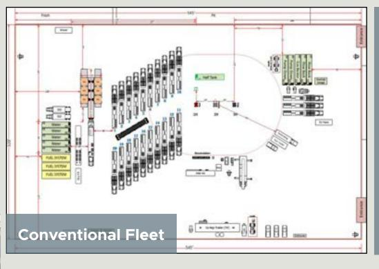
**Simulfrac vs. Conventional Fleet setup:** A simulfrac Fleet rig ups almost twice as much equipment as a conventional fleet - i.e., 2 wireline trucks, 2 cranes, 2 pump down spreads, 2 silo packages and approximately 50% more HHP as shown in the pad layouts below. This allows a SF fleet to pump 2 wells at the same time at a combined rate of 150 bpm vs the standard 100 bpm with a conventional fleet.
